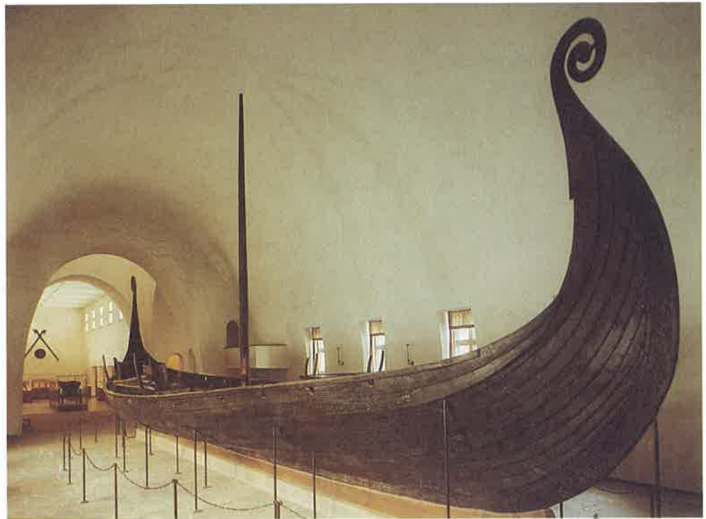
Figure 1-15 Almost 25 metres long, 5 metres wide, and 2 metres deep, this typical ninth-century Viking ship could carry a crew of thirty-two and sail into water just over a metre deep. In 1893, a small crew sailed a replica of a Viking ship across the Atlantic Ocean.
